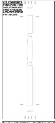
Four (4) ea. #10 x 1%" Stainless Steel "Matching Color" Pan Head Screws. Two each for top and bottom.
