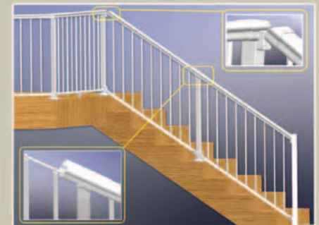
Channelled stair rails, baluster spacing blocks and adjustable baluster knuckles allow for 0-45° angle adjustability
